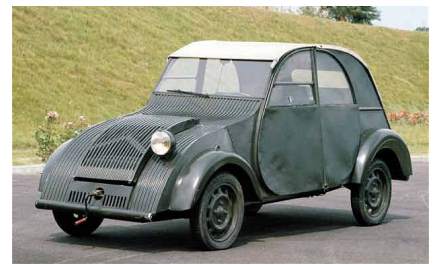
One of the prototype 2CVs Note the single headlight, as required by French law at the time
